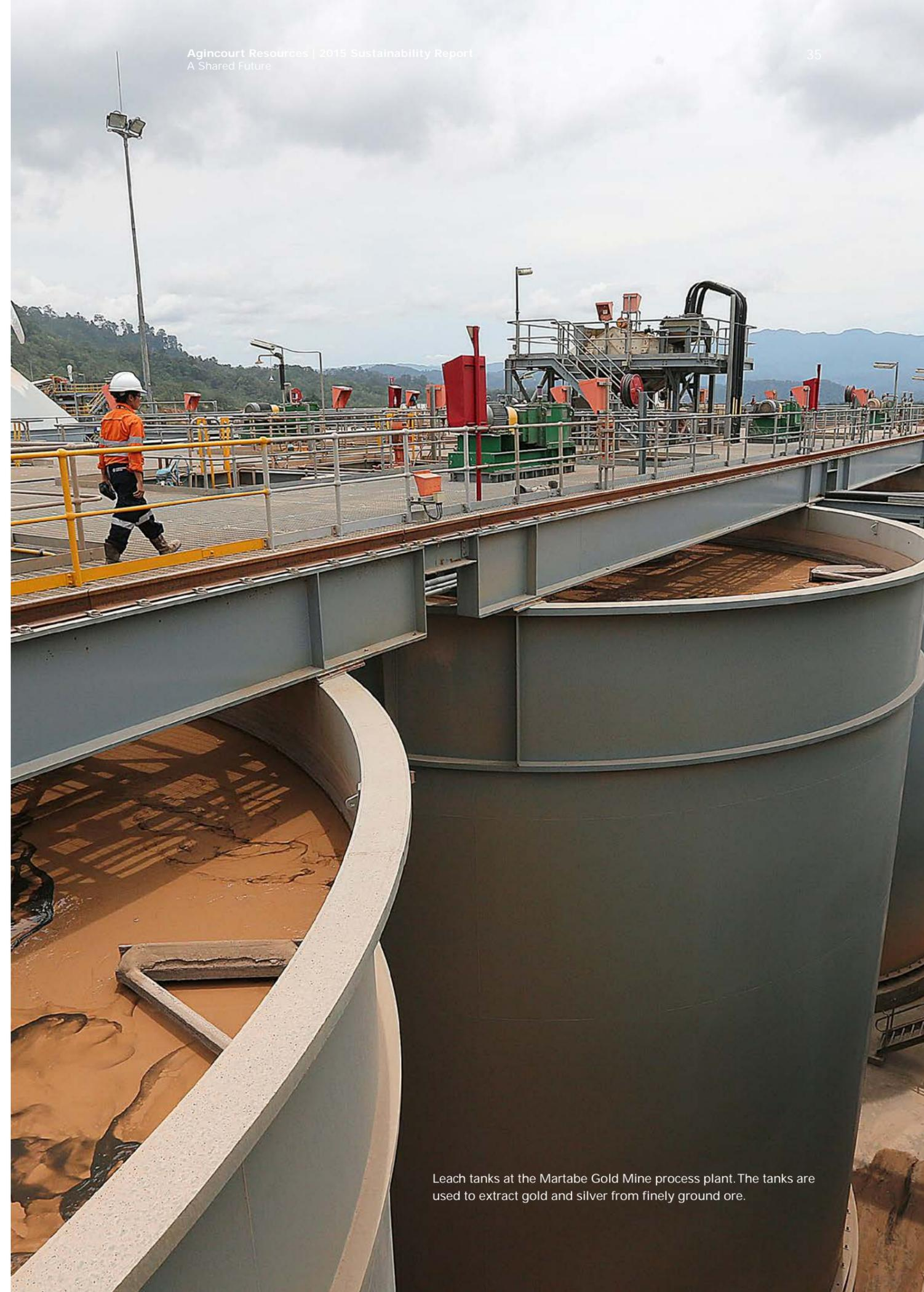
Leach tanks at the Martabe Gold Mine process plant. The tanks are used to extract gold and silver from finely ground ore.
