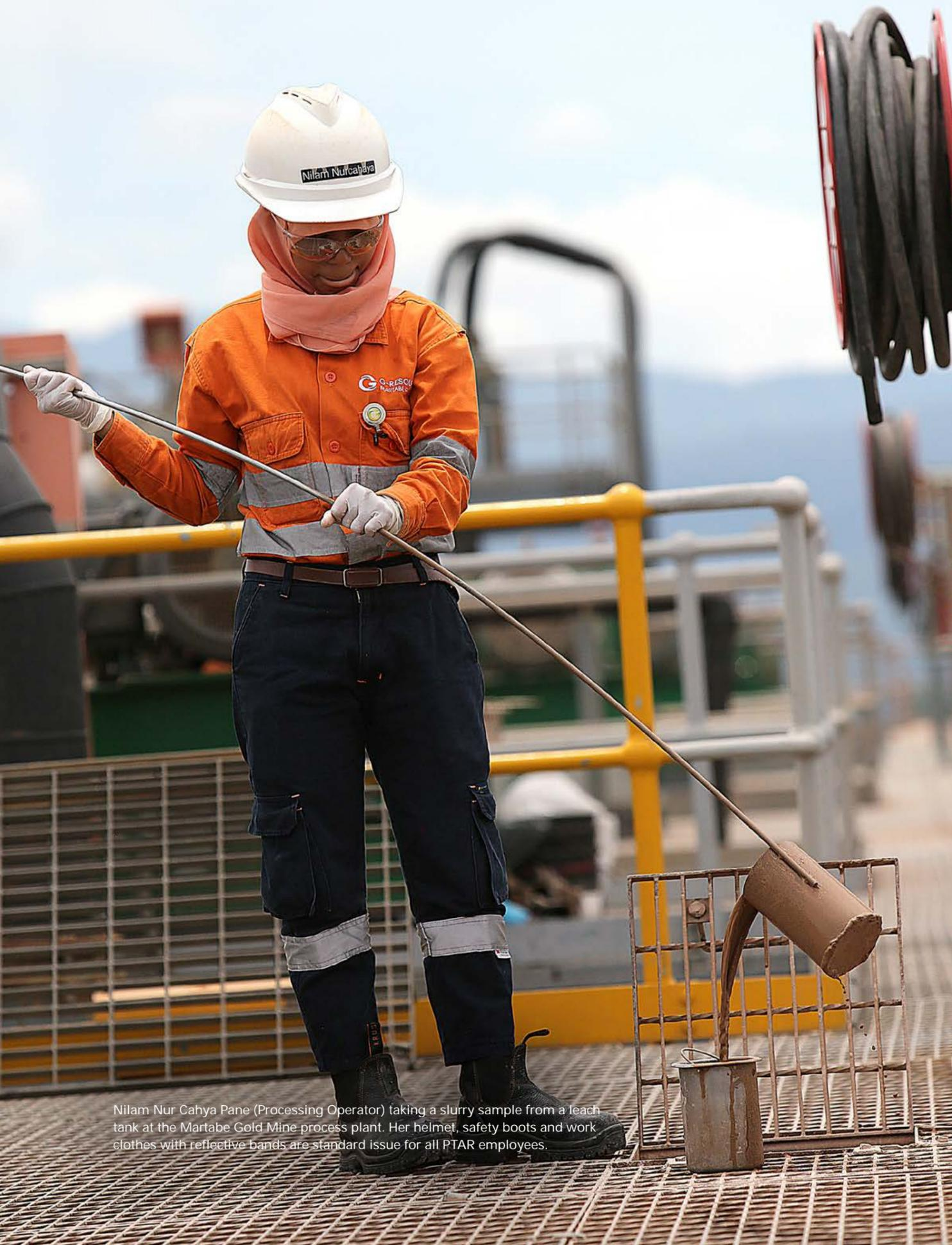
Nilam Nur Cahya Pane (Processing Operator) taking a slurry sample from a leach tank at the Martabe Gold Mine process plant. Her helmet, safety boots and work clothes with reflective bands are standard issue for all PTAR employees.
