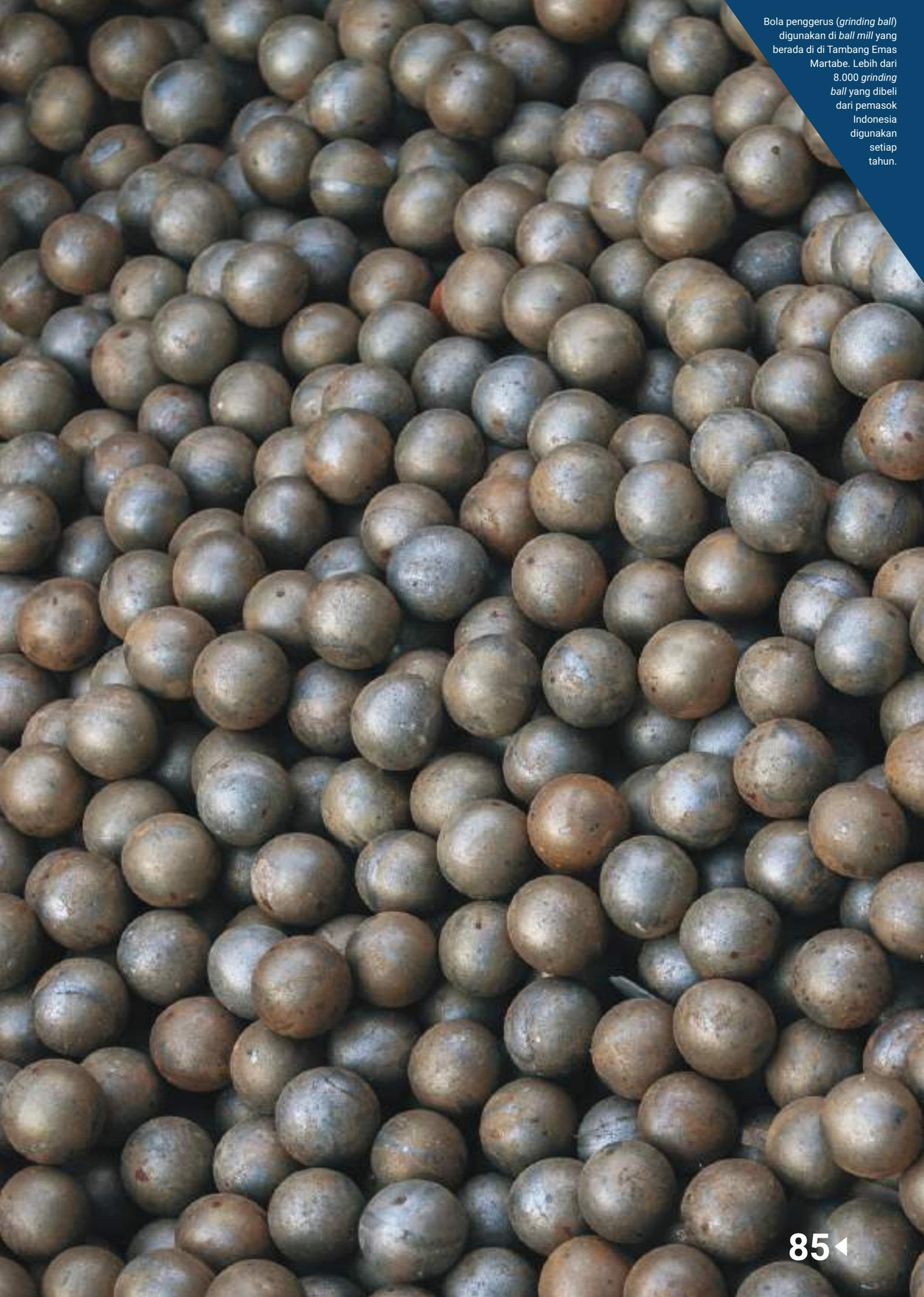
A large pile of used, greyish-brown grinding balls, likely made of steel or iron, filling most of the frame. The balls are spherical and show signs of wear, with some darker spots and a slightly rough texture. They are piled together, creating a dense, textured surface.
