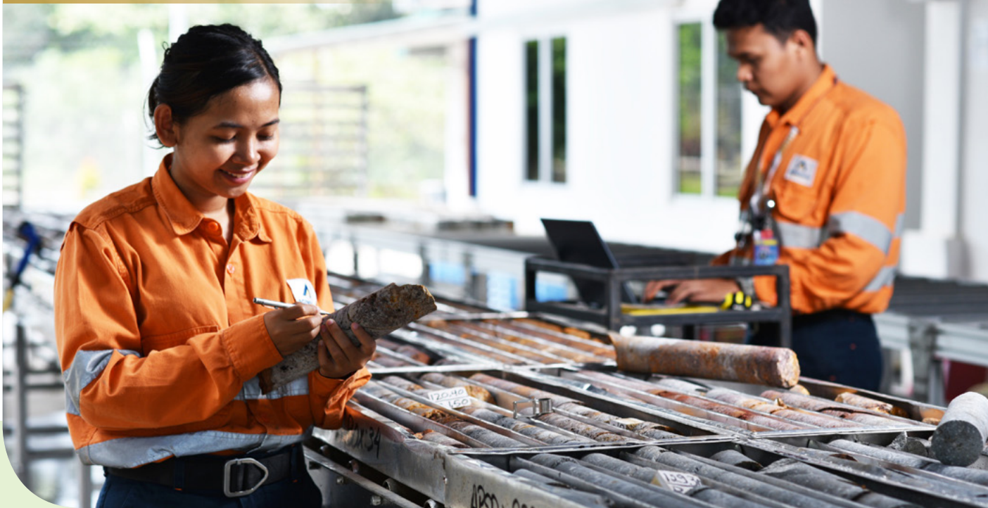
Salma Masti and Ardiansyah Marbun are doing a description of the drilling core rock.
