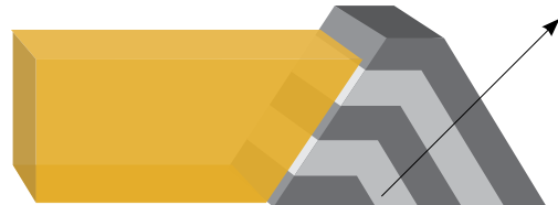
Downstream lifting using engineered compacted zones of rock, clay and sand.
