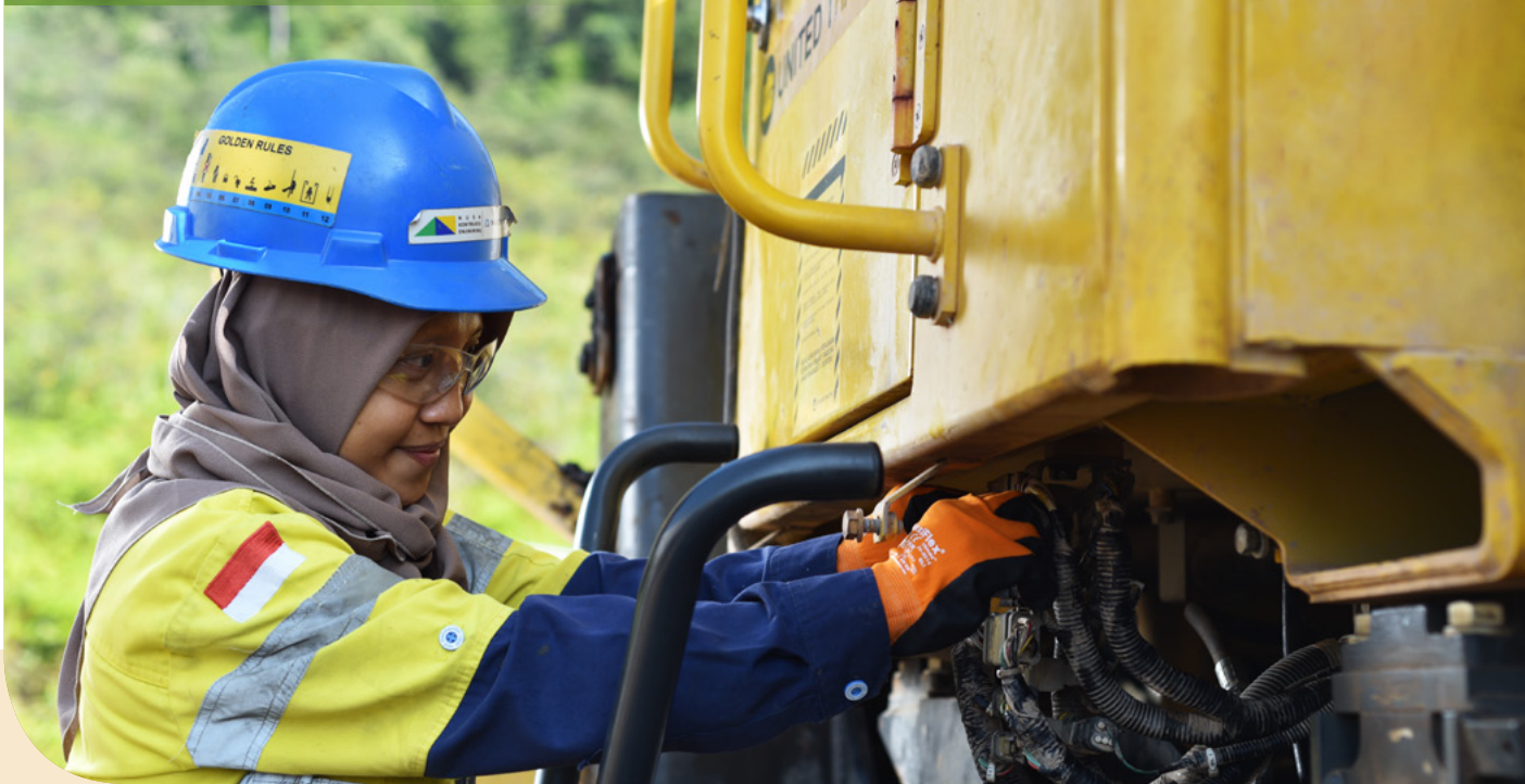
Syafitri Khairunisa (PTAR Contractor) checking the electric system of a wheel loader.
