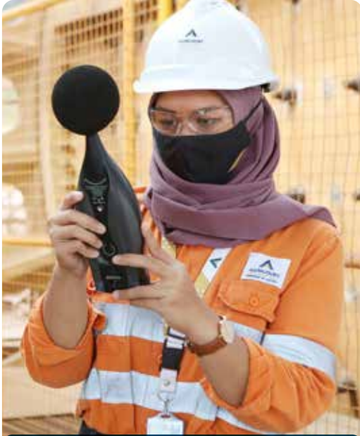
Safety Supervisor, OHS Triana Primadewi is using a sound level meter to measure and ensure the level and control of noise risk around the Martabe Gold Mine operational/work area.
