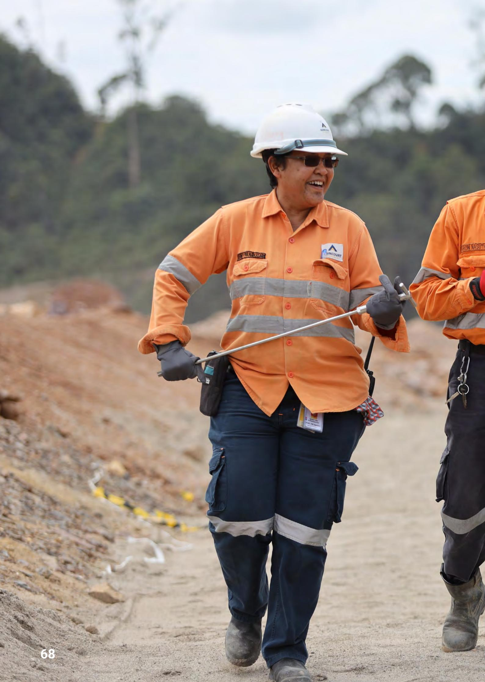
Henny Purnamasari (PTAR TSF Manager), Aron Nasution (PTAR Technician) and Sujarwedi (McMahon JV Surveyor) conduct shear-strength testing at the TSF embankment. Shear-strength is one of a range of parameters that are routinely tested to ensure that the TSF embankment is being constructed to specification.
