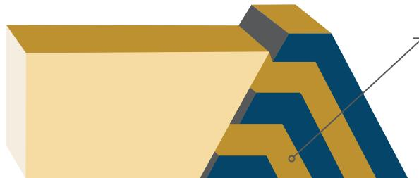
Downstream lifting using engineered compacted zones of rock, clay and sand
