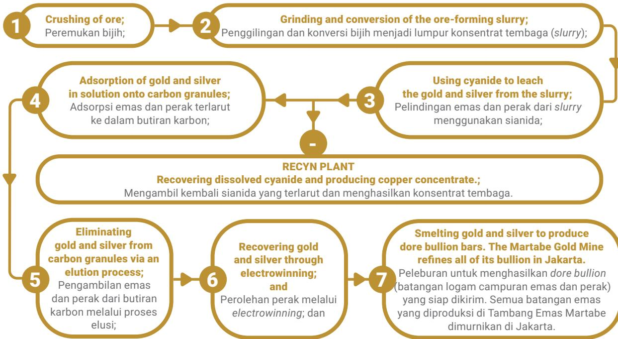
After the gold and silver are extracted from the slurry, the remaining material which is also called tailings will be sent to the ReCyn Plant to extract cyanide and part of the copper. Next, the tailings will undergo a detoxification process. The detoxification process reduces the cyanide concentration to a safe level according to the applicable laws and regulations. In the final stage, the tailings are then transferred to the Tailings Storage Facility (TSF) for safe and permanent storage.
