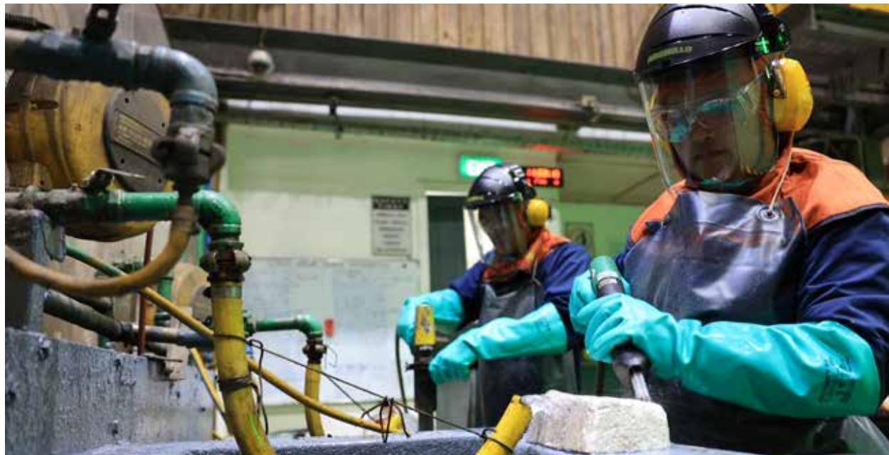
Before entering the stamping stage in the Gold Room, a Clean Bar activity is carried out, namely cleaning the dore bar to ensure that the gold surface is free from residue and ready to be given an official identity as part of the final product quality control.
